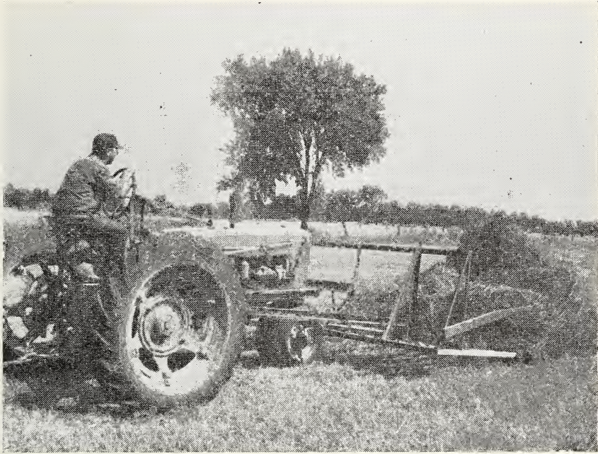
FIGURE 9.—Tractor buckrakes are used to transport hay from windrows to barn or to stack. When the physical lay-out of a farm permits buckraking hay to the barn, it is an efficient and quick way of moving loose hay. The average performance of this type of buckrake, operated by 1 man, was 1.6 tons hauled per hour.
